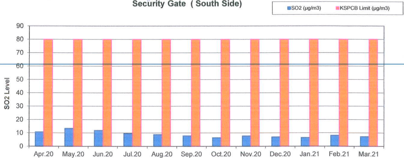
Fig-4: Variation in SO 2 levels from April 2020 to March 2021 Near Materail Security Gate (South Side)
