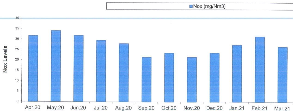
Fig-01: Variation in emission of Nox Levels of stack attached to DG set (1500KVA) from April 2020 to March 2021
